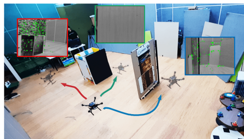
Fig. 2: For robust visual navigation, an aerial vehicle should decide on a path that can guarantee enough visible features from multiple path candidates.(Source: [5], ©2021 IEEE.)
